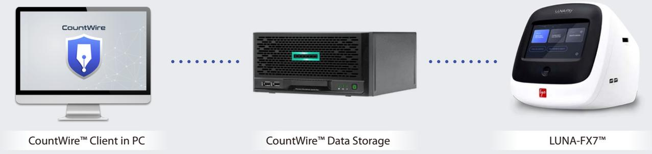
The CountWire™ System consists of the CountWire™ Client software installed in PCs, the CountWire™ Data Storage, and the LUNA-FX7™ Automated Cell Counter, connected and controlled under the same network.
