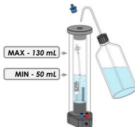
Use a wash bottle to fill the humidifying column. Don't exceed 130 mL. Don't let the water fall below 50 mL during use.
