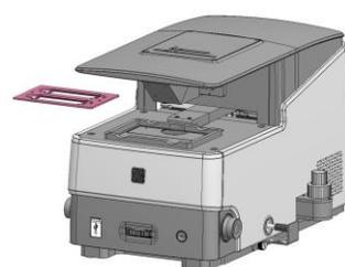
3. Place the desired vessel holder into the vessel holder frame.
