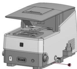
1. Unscrew the screw from the selection tail guard.
