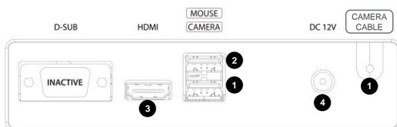
1. Insert the camera cable into the *bottom* USB port.
