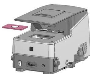
1. Place the insert plate onto the stage with the flat side up.
