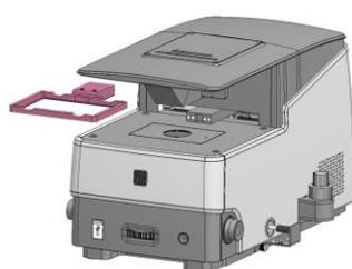
2. Attach the vessel holder frame to the vessel holder frame arm. The frame will snap into place.
