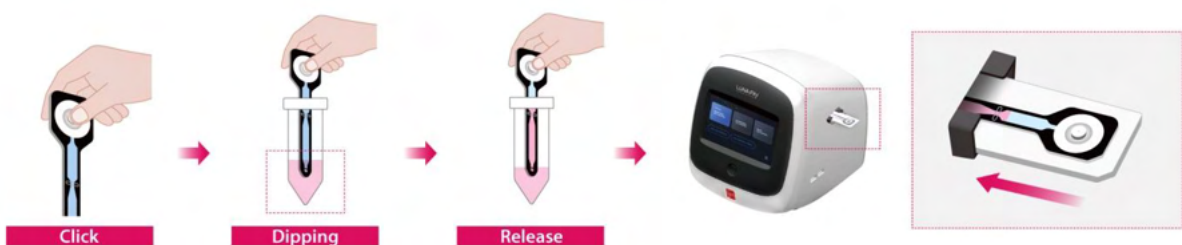
Figure 1. Illustration of the SpectraSlide® AP-1 workflow. Press the sampling button, dip the sampling hole in the sample, release to draw in the liquid, and insert the slide into the LUNA-FX7™ for automated cell counting.
