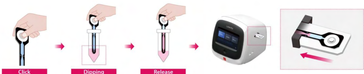
Figure 1. Illustration of the SpectraSlide® AP-1 workflow. Press the sampling button, dip the sampling hole in the sample, release to draw in the liquid, and insert the slide into the LUNA-FX7™ for automated cell counting.
